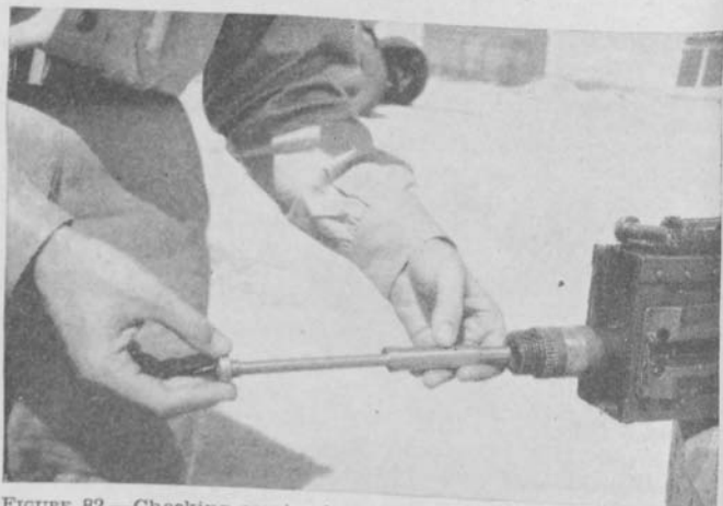
FIGURE 82.—Checking serviceability of a barrel using a bore gage.
