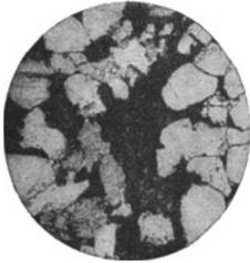
Fig. 12. Eisenschlüssiger Sandstein (Mt. Victoria, New South Wales).
