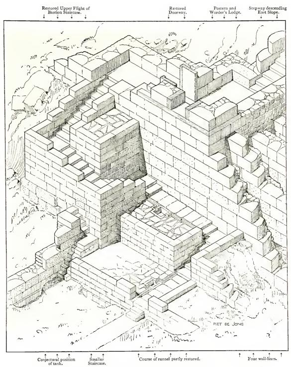
Fig. 166. Isometric Projection of East Bastion and Postern: by Piet de Jong.
