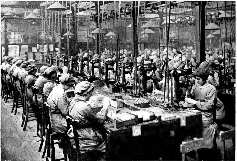
Women Workers and the War: drilling and assembling operations on fuses (Copyright of the Ministry of Munitions)
