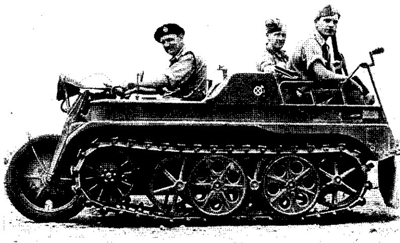
Figure 5. —Captured German half-track vehicle ( Kettenkrad ) frequently used for transport by mountain troops.
