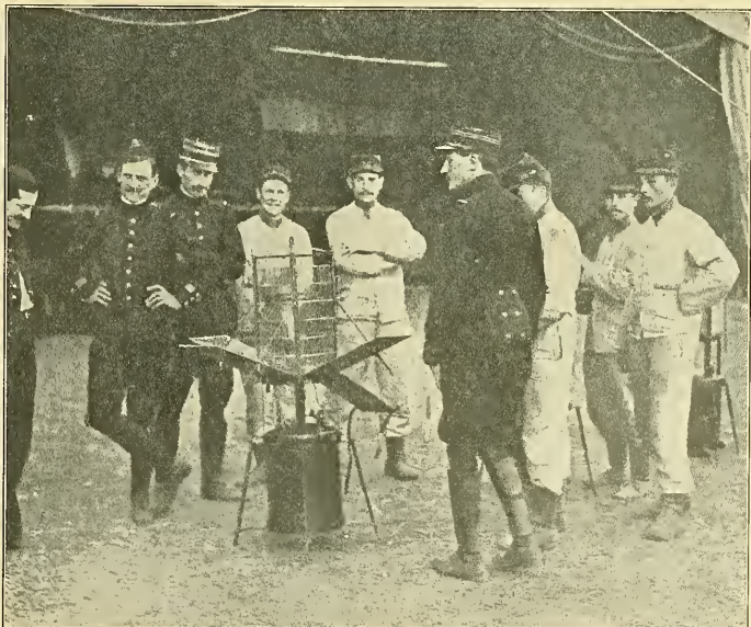
Portable "Lighthouse" for use in directing aviators in night flights. The light is supplied by an acetylene lamp and the rays are thrown upward through a series of lenses and are prevented from spreading by the use of the four blades which revolve around the lenses. The apparatus is the invention of a French officer.
