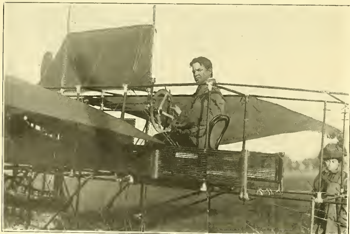
WALTER LOWE FAIRCHILD AT THE WHEEL OF HIS TWIN-PROPELLER MONOPLANE. THE PICTURE SHOWS CLEARLY THE POSITION OF THE EMERSON ENGINE, WHICH IS PLACED LOW WITH THE IDEA OF OBTAINING STABILITY. DESCRIPTION AND DRAWING OF THIS MACHINE FIGURE ON PAGE 134, VOL. 1.
