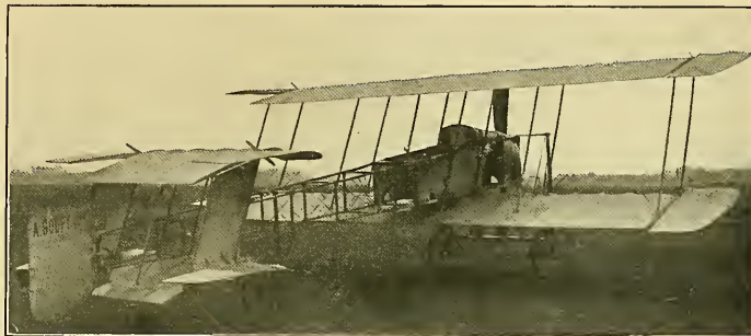
THE SUCCESSFUL GOUPE BIPLANE. NOTE THE BLERIOT FRAME WITH SHORT SKIDS IN FRONT, THE STAGGERED BIPLANE WINGS, THE REAR TAIL, AND NOVEL ALERONS.
