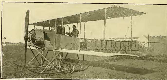
Mr. James V. Martin seated at the control of the new Queen-Martin biplane, which was constructed by the Queen Aeroplane Co. to his designs. The machine is fitted with a 100 H. P. Gnome and carries sufficient fuel for a non-stop flight of 5 hours. Note the strong landing chassis, position of tanks, ailerons on upper surface and flat non-lifting tail.
