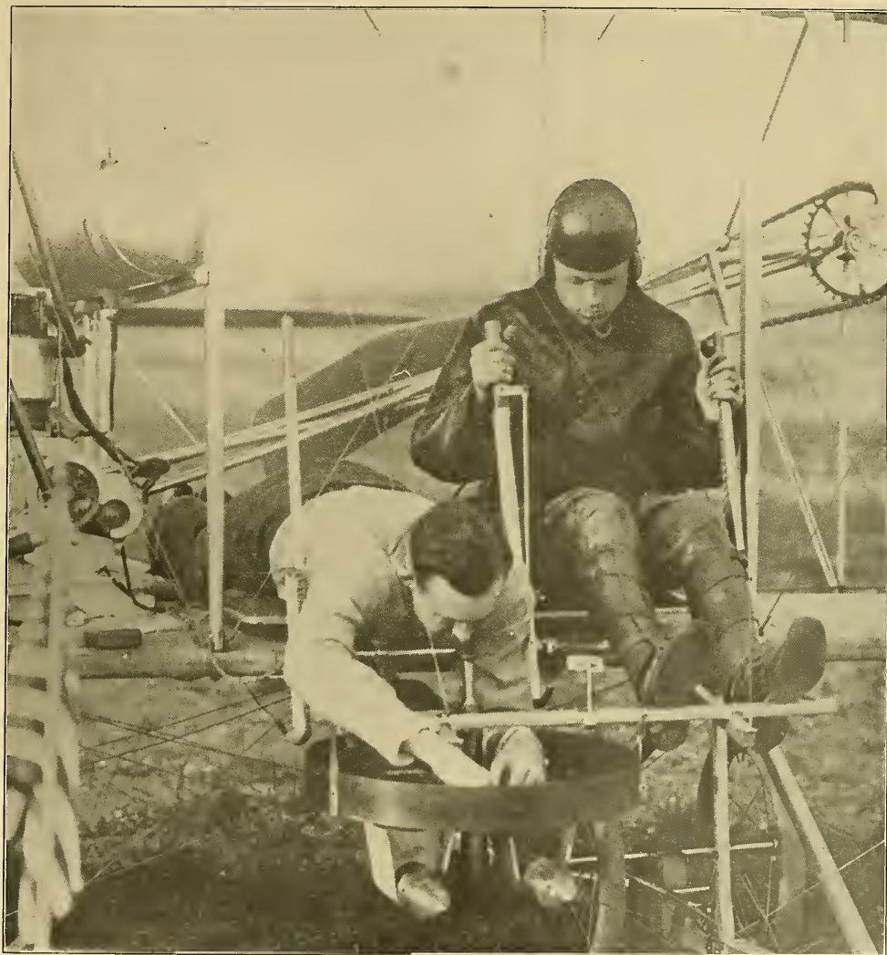
LIEUT. SCOTT ADJUSTING HIS BOMB DRIPPING DEVICE BEFORE STARTING ON A TEST FLIGHT IN AN ARMY BIPLANE, WITH LIEUT. MILLING AS PILOT
