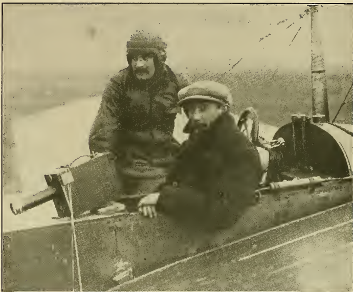
A VIEW SHOWING THE SEATING ARRANGEMENTS OF THE 100 H. P. DEPEROUSSIN MONOPLANE AND KINETOGRAPH IN POSITION READY TO TAKE PICTURES.
