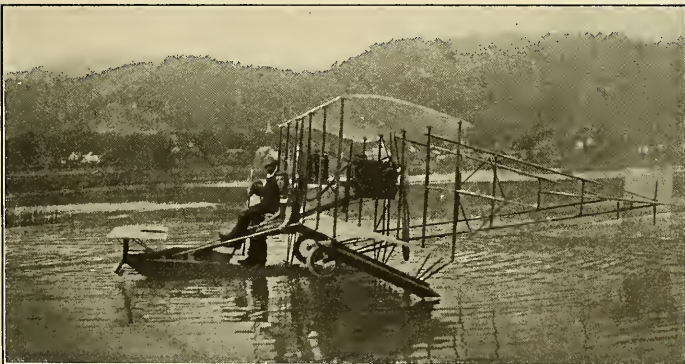
Glenn H. Curtiss and Lieut. Ellyson, U. S. N., just after alighting upon the lake at Hammondsport, N. Y., after making a fine flight in his latest hydro-aeroplane. This machine is built to run along the ground, alight on the water or fly in the air.
