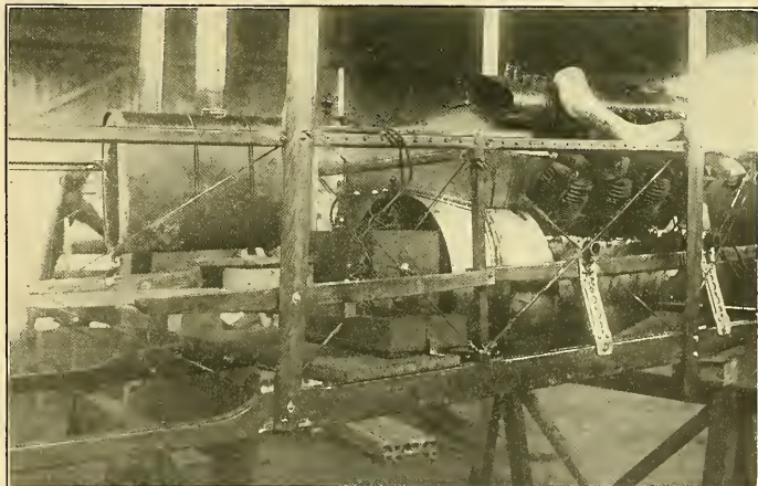
A WIRELESS INSTRUMENT INSTALLED ON A MAURICE FARMAN BIPLANE. IN TRIALS AT THE BUC AERODROME MESSAGES WERE SENT FROM THE BIPLANE WHILE IN FLIGHT AND WERE SUCCESSFULLY CAUGHT BY THE RECEIVING APPARATUS LOCATED IN THE SCHOOL WORKSHOP. THE PHOTOGRAPH ALSO SHOWS THE INSTALLATION OF THE RENAULT MOTOR.
