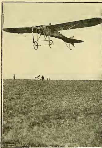
THE LATEST SINGLE-SEATER BLERIOT. NOTE THE TAPERING FRAME, FLAT TAIL AND TRIANGLE-SHAPE RUDDEERS.
