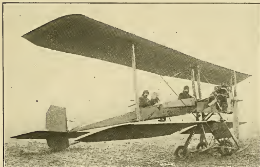
THREE-QUARTER VIEW OF TWO-SEATER MILITARY TYPE BREGUET SHOWING POSITION AND MOUNTING OF THE R. E. P. MOTOR.
