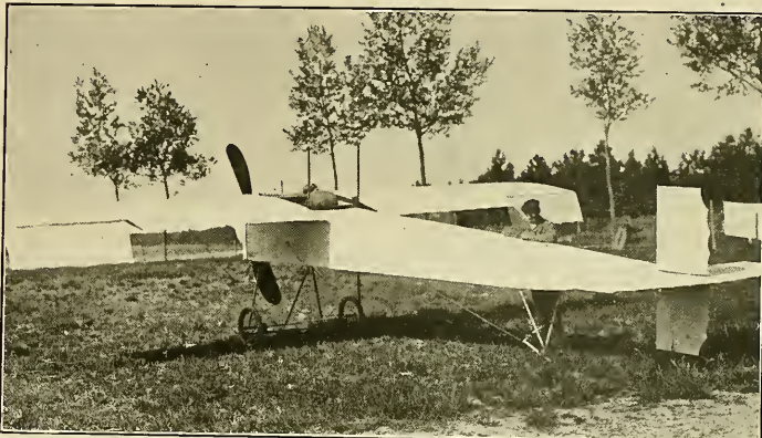
The above photograph shows the cruciform tail comprising the elevator and rudder. On the trailing extremities of the main wings are hinged balancing ailerons. The span of the machine is 9 metres (nearly 30 feet) and the over all length 8 5/10 metres (28 feet). The starting area is 17 sq. metres (about 183 feet).
