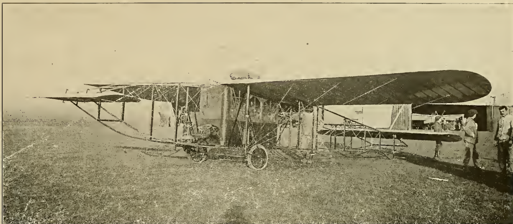
The above is a three-quarter view of the latest Blériot Aerocar built to the order of Henri Deutsch (de la Meurthe). The inside is fitted as luxuriously as a limousine automobile and is made to seat four persons besides the driver, who sits in front on the outside. The seats are made with air cushions in order to break the shock in case of rough landing. There is a door on each side and windows of a transparent non-brittle material on three sides, so that the passengers may have a good view of the surrounding country as they speed along. According to Legagneux—who has been experimenting with this machine—it works as well as any of the other Blériot styles.
