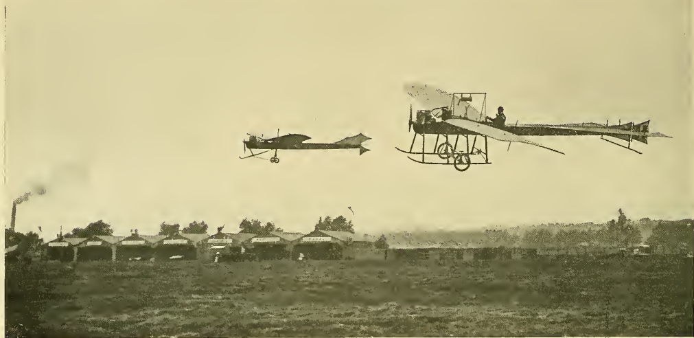
A RACE BETWEEN THE HANRIOT AND ANTOINETTE MONOPLANES. THE MACHINE ON THE RIGHT IS THE HANRIOT. NOTE THE BOAT-SHAPED HULL, FLAT TAIL, A TYPE CHASSIS AND COMBINATION WHEELS AND SKI LANDING GEAR.
