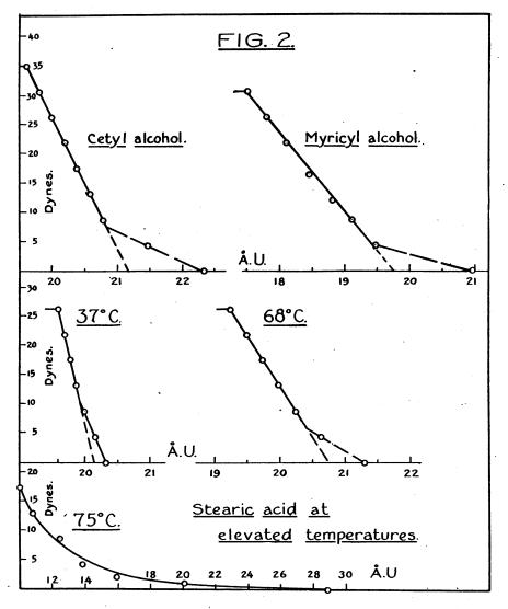
the curve shows that the film is extremely weak. It should be mentioned that the value of the compressive force at collapse depends somewhat upon the rapidity of compression.
