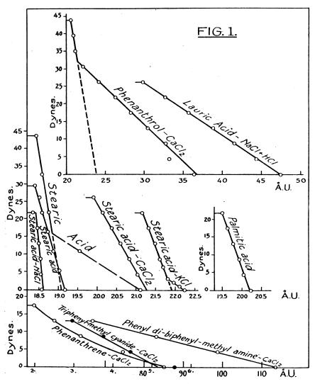
Polymolecular Films.—Phenanthrene spread on an aqueous calcium chloride solution gives a typical polymolecular film. Though this substance has a large molecule (14 carbon atoms and 10 hydrogen atoms), the zero area is very small: only 5.6 A.U., with a thickness of 47Å which
