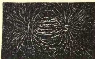
FIG. 34.—DISTRIBUTION OF FLUX BY CUT IRON WIRE IN PLANE OVER POLES OF ELECTRO-MAGNET.
