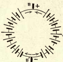
FIG. 102.—VOLTAIC ANALOGUE OF E. M. Fs. GENERATED IN GRAMME RING.
