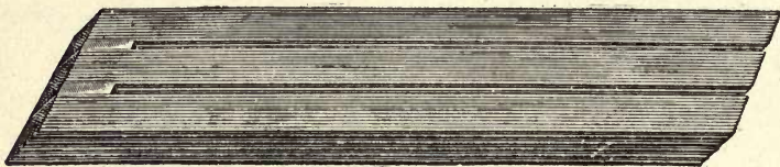
FIG. 106.—FORM OF GENERATOR BRUSH.
