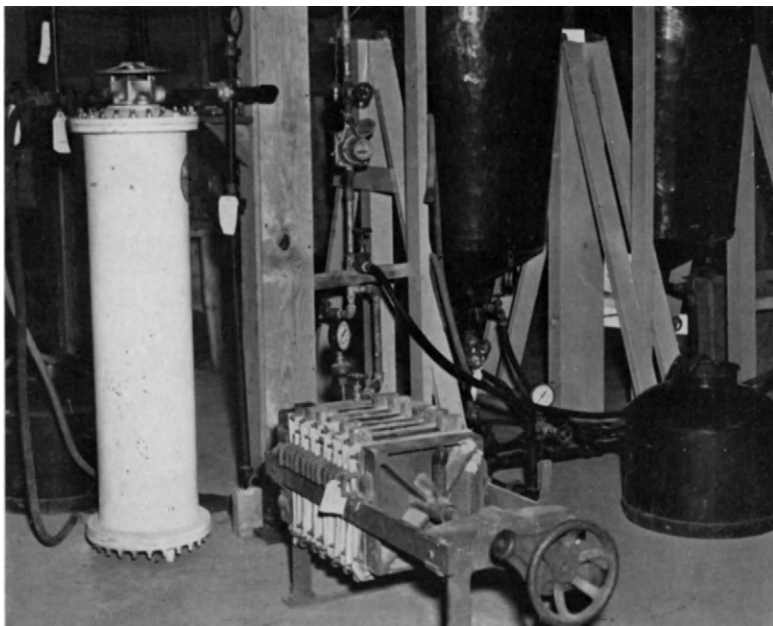
FIG. 1. Cyclic ion exchange plant for the recovery of scopolamine (from Chem. Inds. 57 , 455, 1945).
