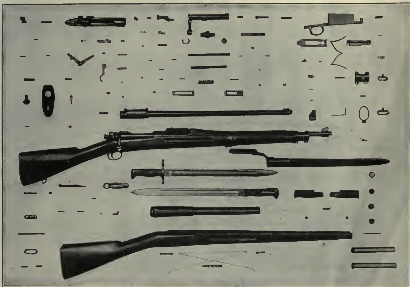
FIG. 1. SAMPLE BOARD, SHOWING VARIOUS PARTS OF SPRINGFIELD MODEL 1903 SERVICE RIFLE
