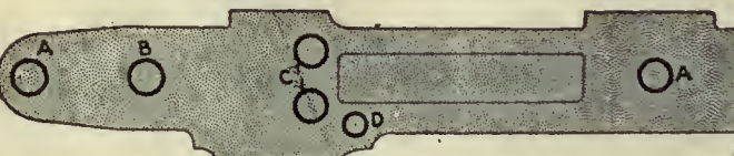
AA-Guard Screws, B-Sear Nose, C-Rear of Magazine, D-Ejection Pin
