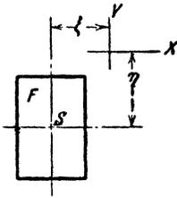
$$J_{xy} = F \xi \eta \dots \dots \dots 30$$
