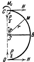
worin  $\frac{\delta M}{\delta M_C} = 1$ ,  $\frac{\delta S}{\delta M_C} = 0$ ;  $\frac{\delta M}{\delta H} = r(1 - \cos \varphi)$ ,  $\frac{\delta S}{\delta H} = 2$
