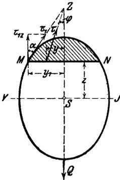
Randspannung:  $\tau_1 = \frac{\tau_{1z}}{\cos \alpha} \dots \dots 99$
