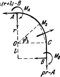
$$M = M_C - \int_{\psi=0}^{\varphi} q \, ds \cdot r (\sin \varphi - \sin \psi) = M_C - q r^2 (\varphi \sin \varphi + \cos \varphi - 1).$$
