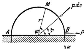
$$M = Kr(1 - \cos \varphi) - Pr \sin \varphi + \int_0^\varphi p ds \cdot r \sin(\varphi - \psi), \quad ds = r d\psi,$$
