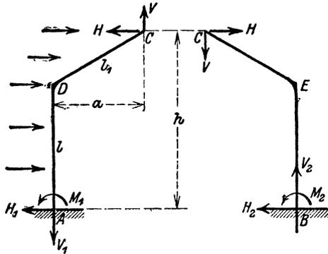
$$A_1 = \frac{1}{2EJ} \int_0^l \left( -M_1 + H_1 x - \frac{q x^2}{2} \right)^2 dx + \frac{V_1^2 l}{2EF},$$
