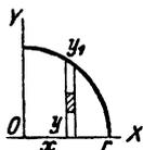
$$\begin{aligned} 145. \quad J_{xy} &= \int \int xy \, dx \, dy = \int_0^r [x dx \int_0^{y_1} y \, dy] \\ &= \int_0^r x \, dx \cdot \frac{y_1^2}{2} = \frac{1}{2} \int_0^r x \, dx \cdot (r^2 - x^2) = \frac{r^4}{8}. \end{aligned}$$
