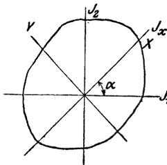
$$\left. \begin{aligned} J_x &= J_1 \cos^2 \alpha + J_2 \sin^2 \alpha \\ J_{xy} &= (J_1 - J_2) \sin \alpha \cos \alpha \end{aligned} \right\} \dots 28$$
