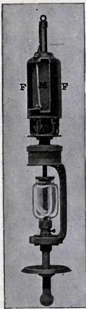
FIG. 46.—FORM OF ARC LAMP FOR CONSTANT-POTENTIAL CIRCUITS, SHELL AND OUTSIDE GLOBE REMOVED.
