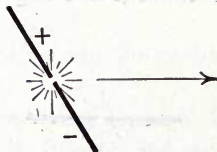
FIG. 7.—ARRANGEMENT OF CARBONS FOR USE IN A PROJECTOR.
