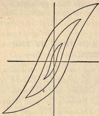
Fig. 11B. Hysteresis Loops with Various Maximum Magnetic Inductions in the same Iron.
