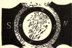
Fig. 181 Cause of Lead of Brushes.
