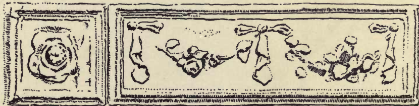
EXTERNAL PLASTER DETAILS (PARGETTING) FROM HERTS, ESSEX, AND SUFFOLK
