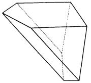
Fig. 26.-Amici's 'roof' prism.
