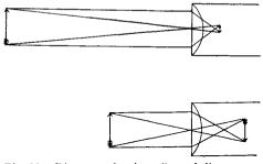
Fig. 11.—Diagrams showing effect of distance on the size of the resultant image.
