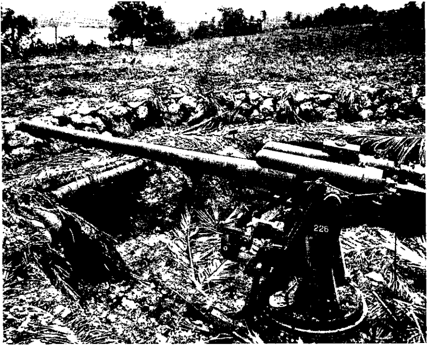
Figure 58.—Model 10 (1921) 120-mm dual-purpose gun. Note revetment details and ammunition storage.
