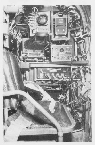
(1) Indicator BC-929-A (2) Radio Control Box BC-1145-A
