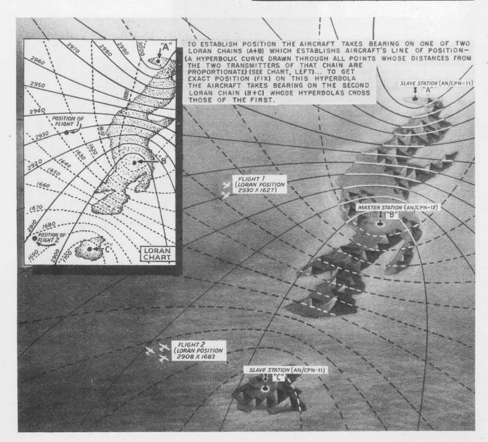
Radar Set AN/CPN-12 and AN/CPN-11 constitute an air transportable ground Loran chain which provides properly equipped aircraft with means whereby they may obtain a fix of position at any time within the range of 200 miles by day and 400 miles at night.
