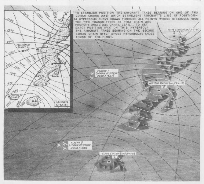
Radar Sets AN/CPN-11 and AN/CPN-12 constitute an air transportable ground Loran chain which provides properly equipped aircraft with means whereby they may obtain a fix of position at any time within the range of 200 miles by day and 400 miles at night.
