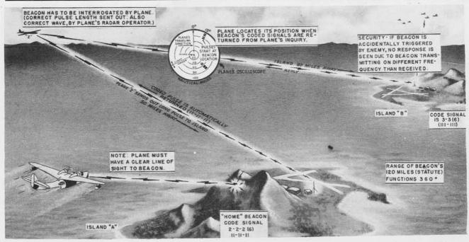
Radio Set AN/CPN - 8 is an Air Transportable Radar Beacon designed to provide range, direction, and identification for homing 10 cm band radar equipped aircraft.
