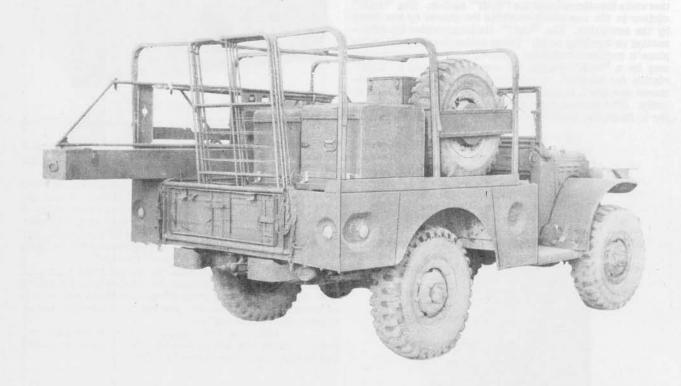
Complete installation of Vehicular Mounting Kit for Radio Set AN/CPN-2.
