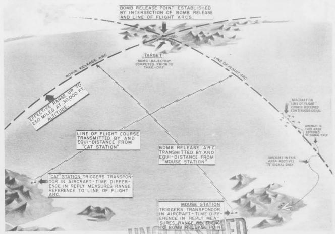
Radar Assembly AN/APA-9 ("ASPEN") is the airborne element of the OBOE Navigation System which in addition to facilitating precision blind bombing - may be used as a navigation device to direct reconnaissance or troop carrying aircraft to predetermined areas.
