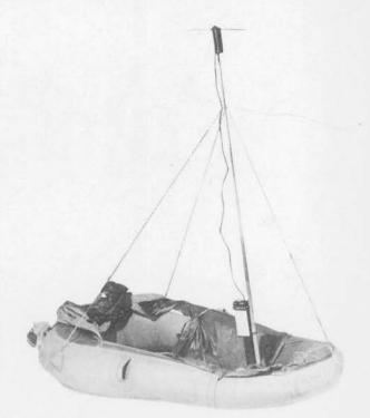
Radio Set AN/CPT-2 is installed in life raft after being forced down and operates automatically.
