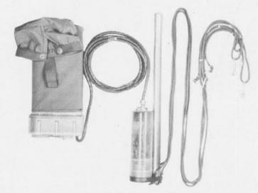
Components of Radar Beacon AN/CPN-16
