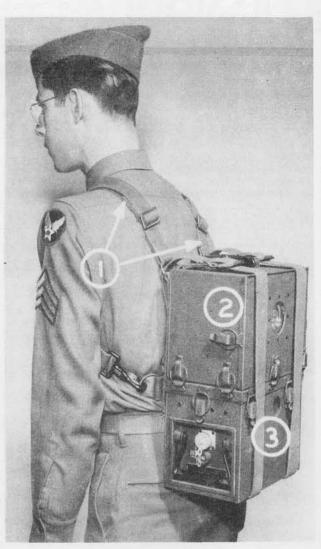
Battery Charger & Battery in carrying position-entire equipment may be packed in 2 packages & carried by one man. (1) Harness MX-253/UPN-1 (2) Rectifier Battery Charger PP-116/UPN (3) Battery Case CY-222/UPN-1.
