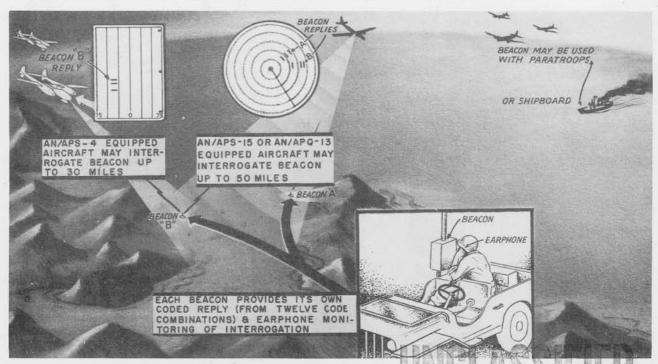
Radar Beacon AN/UPN-3 (BUPX) is an ultra portable ground, paratroop and shipborne beacon designed to provide navigation information, act as homing beacon and designate bomb runs.
