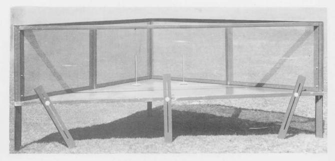
Antenna System AS-30/CPA-1 assembled for operation.
