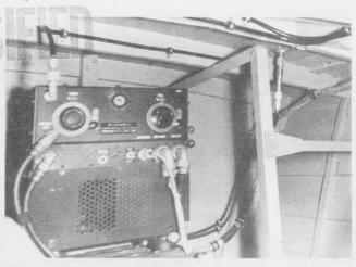
Receiver-Transmitter RT-21/APN-7 installed for operation.
