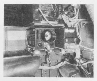
Indicator I-152-() installed in aircraft.
