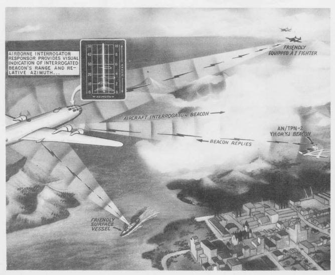
Radar Set AN/APN-12 is an airborne interrogator responsor equipment used in conjunction with ground beacons for aircraft navigation and for Mark III IFF land, sea and air operations.
