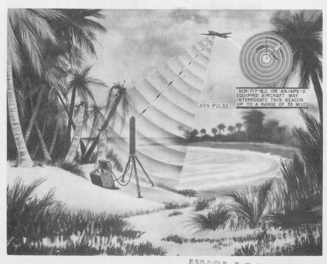
Radar Beacon AN/UPN-2 on being interrogated by airborne radar (on beacon function) replys in code permitting the beacon to be located in range and azimuth. Graphic Survey
