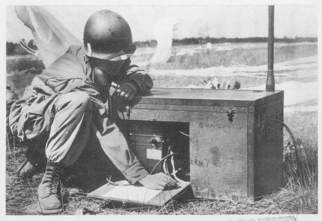
Beacon Transmitter AN/TPN-3 is an air transportable Radar Beacon providing homing facilities to troop carrying aircraft under conditions of poor visibility. Section 4 - Graphic Survey July 1945
