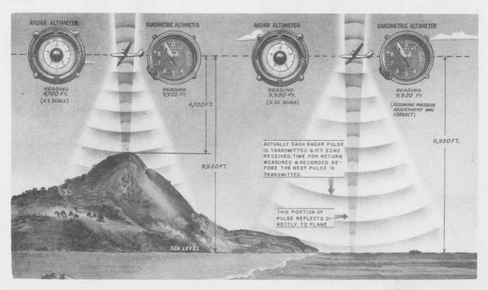
Radio Set SCR-718 is a precision altimeter which records the absolute altitude of an aircraft above the terrain, regardless of air pressure or variations in temperature.
