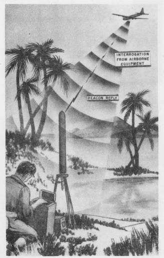
Aircraft Interrogation Triggers Beacon Reply which establishes its identity & position in range and azimuth. July 1945
