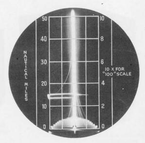
Scope records range vertically on three scales & azimuth horizontally right or left of centerline of beacon response signal above shows beacon 33 miles away & approx.30 right.
