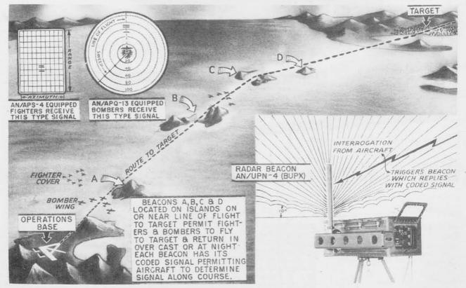
Radar Beacon AN/UPN-4 is an ultra portable ground, paratroop and shipborne beacon designed to provide navigation information, act as homing beacon and designate bomb runs to aircraft equipped with radars operating in its frequency range.
