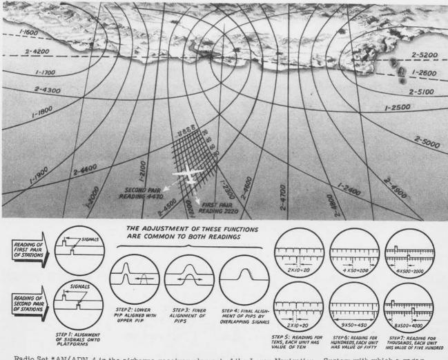
Radio Set \*AN/APN-4 is the airborne receiver element of the Loran Navigation System with which a radar fix is obtained by taking a reading on each of two Loran chains in the order shown.
