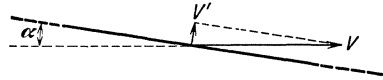
Fig. 74. Normal component of the velocity of approach of a plate of large chord dimension.
