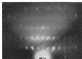
Fig. 45. Haematite: beam grazing intersection of two natural faces.
