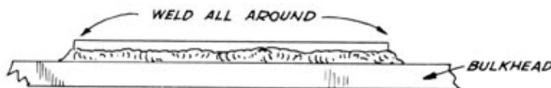
Side View of a Correctly Welded Pad on the Bulkhead of a Ship
