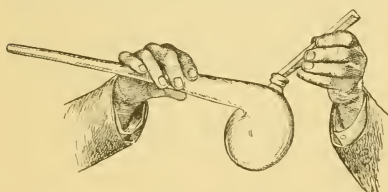
FIG. 101. — Pouring a solid into a vessel with a small opening.
