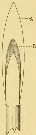
FIG. 71.—The oxidizing ( A ) and reducing ( B ) flames.
