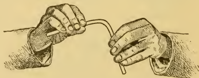
FIG. 6.—Bending a tube into a right angle—II.
