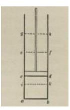
contact of the same temperature as the body A; cd is the actual position of the piston.
