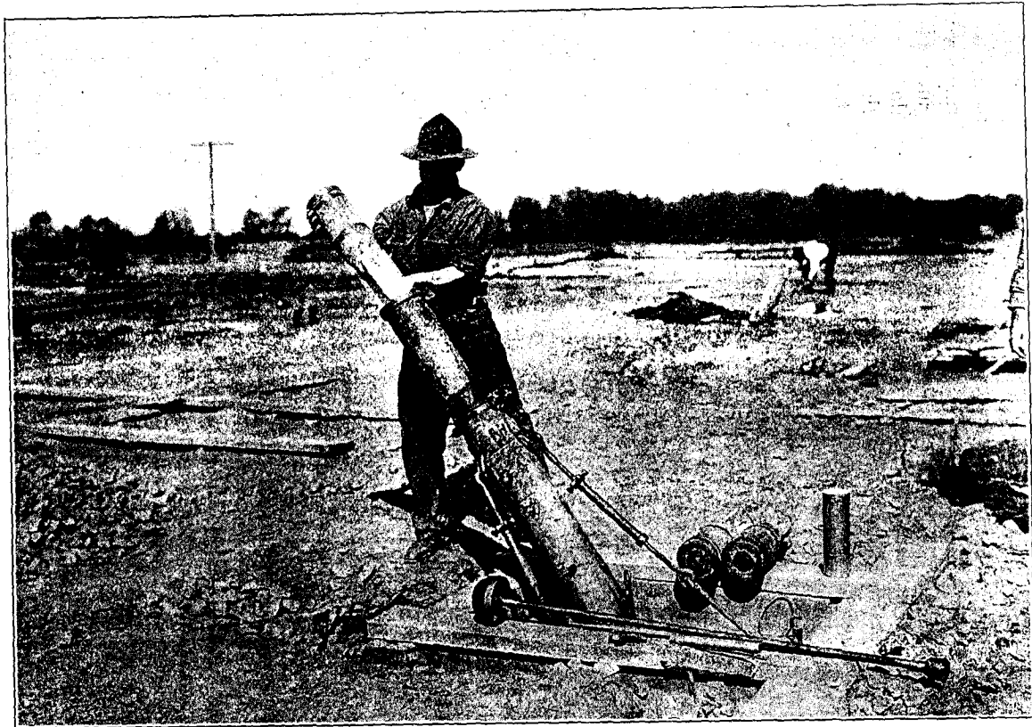
FIG. 98.—6-inch trench mortar. Loading projectile and charge. Note in the foreground gas ejector employed as a piston to expel gases after a discharge.
