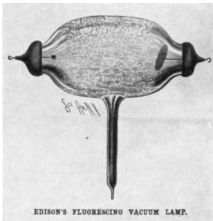
Abb. 81. EDISON'S fluoreszierende Vakuum-Röntgenlampe. (Aus Electrical Engineer 21, 378, 15. April 1896).
