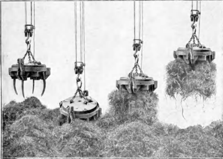
Fig. 15 Scrap hoisting by means of cranes with magnets attached to them
