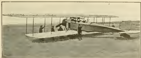
The Schmitt biplane of varying speed which can go at over 100 kilometers an hour as well as 39 kilometers an hour. With this machine Garaix recently carried 6 passengers 107 kilometers (66½ miles) in one hour as well as on different occasions, making a number of World's records for altitude with passengers.
