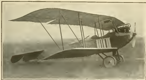
The 100 h.p. Mercedes aviatik-pfeil biplane with which Ingold, the German aviator broke the world's duration record by remaining in the air over 16 hours. See March AIRCRAFT, Page 279.
