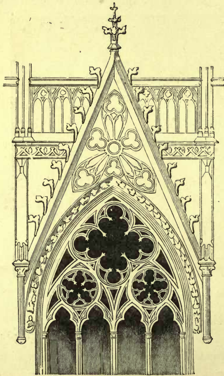
FIG. 100.—Window, gable, and parapet, in Cologne Cathedral.
