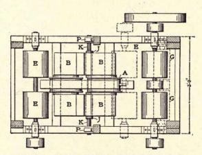
FIG. 49. - WETHERILL INCLINED SEPARATOR.
