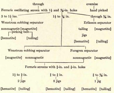
The crude ore carries magnetite, hematite, and pyrites in pegmatite and schistose material. The ore carries about 40 per cent. iron and the concentrate from 60 to 61 per cent. iron. The concentrate is roasted to remove sulphur.
