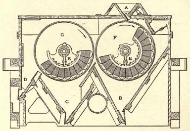
FIG. 2.—THE BALL-NORTON DOUBLE-DRUM SEPARATOR.
