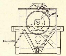
FIG. 16. - THE BALL-NORTON SINGLE-DRUM SEPARATOR.
