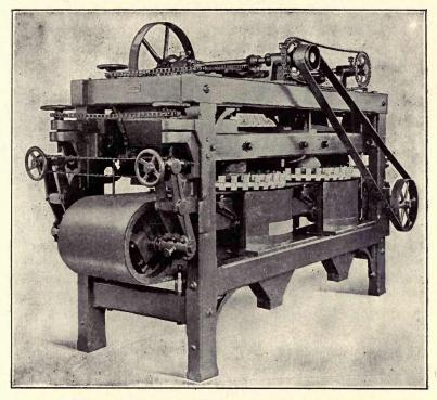
FIG. 19.—THE DINGS BELT TYPE SEPARATOR.
