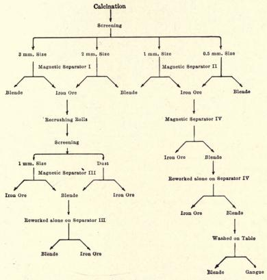
The ore, after calcination, is crushed to pass 4 mm. and then classified into the following sizes: on 3 mm.; on 2 mm.; on 1 mm.; and through  $\frac{1}{2}$  mm. The two larger sizes are treated upon Sep-
