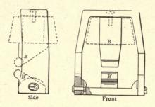
FIG. 31. - DETAIL OF PRIMARY MAGNET, KNOWLES SEPARATOR.
