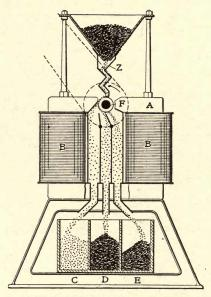
FIG. 8.—THE WETHERILL TYPE F SEPARATOR.
