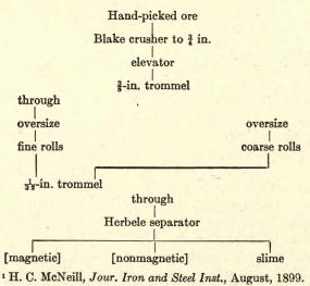
The magnetic product contains the magnetite and pyrrhotite and but little galena and blende. The nonmagnetic product of the separator is concentrated on jigs, tables, etc., and the quartz removed. The overflow from the separator is allowed to settle and the slime, consisting mostly of blende and silica, is treated for zinc.
