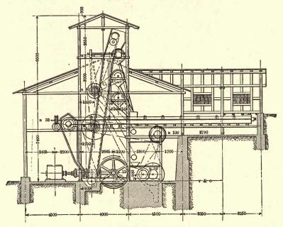
FIG. 66.—TRANSVERSE SECTION OF SEPARATION WORKS, NEUNKIRCHEN, GERMANY,
