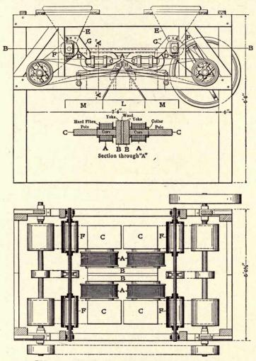
FIG. 48. - WETHERILL HORIZONTAL SEPARATOR.
