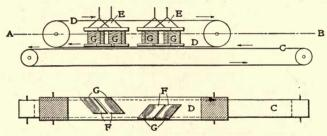
FIG. 47. - WETHERILL PARALLEL SEPARATOR.
