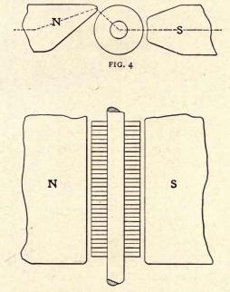
FIG. 9. - DETAILS OF MAGNET ROLLER, WETHERILL TYPE F SEPARATOR.
