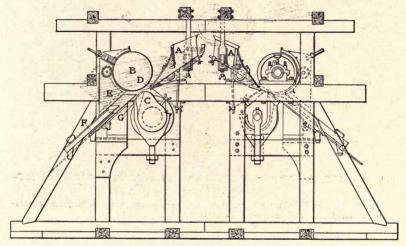
FIG. 37. - MECHERNICH SEPARATOR.
