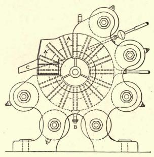
FIG. 22.—THE STERN-TYPE WET SEPARATOR. SIDE ELEVATION.
