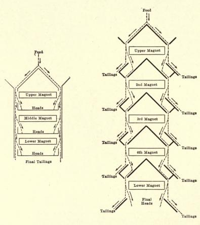
FIG. 13.—PRELIMINARY MAGNETS, EDISON SEPARATOR.
