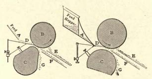
FIG. 36.—CROSS-SECTIONS OF MAGNETS, MECHERNICH SEPARATOR.
