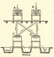
FIG. 68. — ARRANGEMENT OF SEPARATORS, FRIEDRICHSSEGEN, GERMANY.
