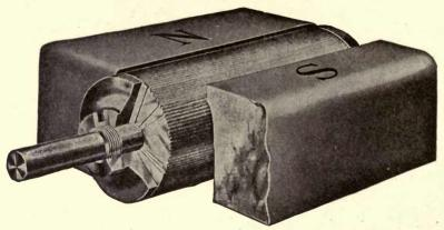
FIG. 42.—DETAIL OF SEPARATING ARMATURE, INTERNATIONAL SEPARATOR.
