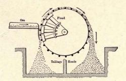
FIG. 28.—THE HEBERLE DRY SEPARATOR.
