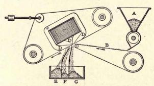
FIG. 46. - HUMBOLDT-WETHERILL TYPE VI SEPARATOR.
