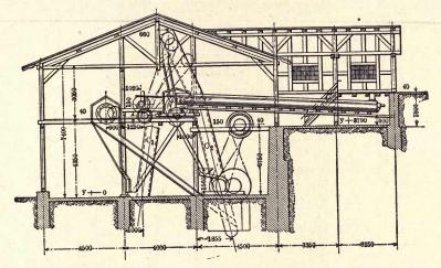
FIG. 65. — TRANSVERSE SECTION OF SEPARATION WORKS, NEUNKIRCHEN, GERMANY.
