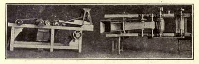
FIG. 27.—THE FERRARIS DRUM SEPARATOR.
