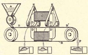
FIG. 32.—SKETCH SHOWING PRINCIPLE OF WETHERILL-ROWAND SEP-ARATOR.
