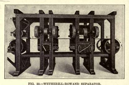
A, Feed hopper; B, feed roller; C, conveyor belt; D, cross belts; E, nonmagnetic discharge.
