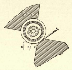
FIG. 38.—DETAIL OF MAGNET POLES AND ARMATURE, MOTOR-TYPE SEPARATOR.
