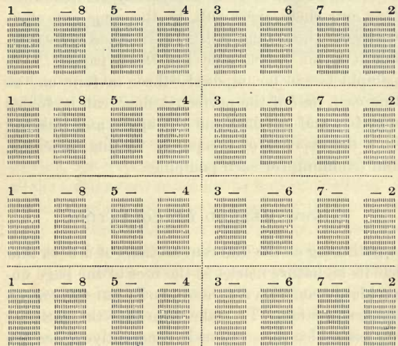
50 Eight pages in quadruplicate, or "four on." Sheet turns on short cross. Produces eight copies.
