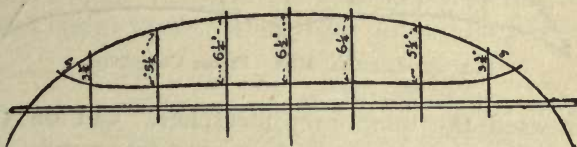
FIG. 53.—Cannibal Kite. Reverse bow bent and fastened in place.
