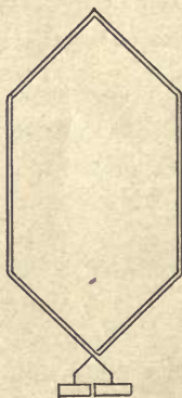
FIG. 76.—Two turn coil for a drum winding.
