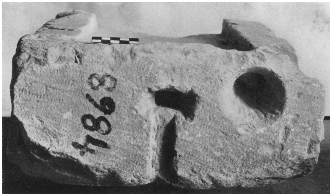
View of the Top of No. I, Showing Hopper and Cutting for the Clamp
