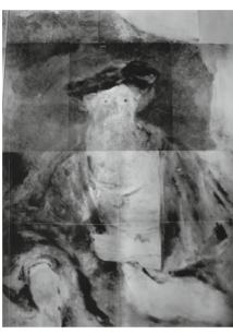
Fig. 2. Neutron-activation autoradiograph of  $\boxed{\textbf{203}}$  The darkest parts showing the phosphorous component of bone-black which may be found in different layers of the painting.
