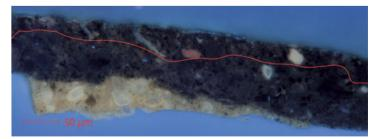
Fig. 7. Cross-section of a sample taken in the signature. The red line indicates the boundary between the paint of the background and the paint of the signature. Microscopic examination shows that the latters contains more black pigment particles.
