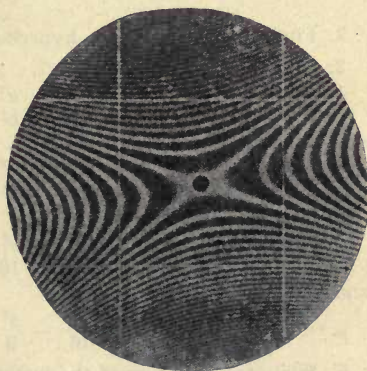
FIG. 80.—A Family of Conjugate Pairs of Hyperbolas with Common Asymptotes. (An interference pattern made from a glass plate under compression. From R. Strauble, "Ueber die Elasticitäts-zahlen und modulen des Glases." Wied. Ann. Bd. 68, 1899, p. 381.)
