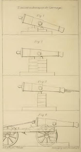
8,9 and 10 draw out the carriage. Nos. 3 and 4 build up the rear seaffold of four blocks on each side, and place the other half roller on top of it, under the reinforce.
