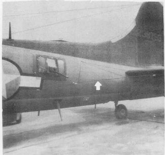
Fan Antenna for Radio Transmitting Equipment AN/ART-3 on B-17.
