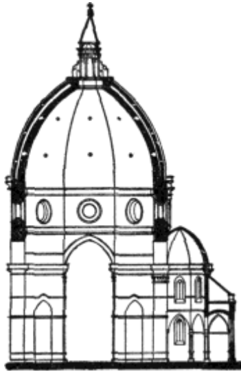
FIG. 159.—SECTION OF DOME OF DUOMO, FLORENCE.
