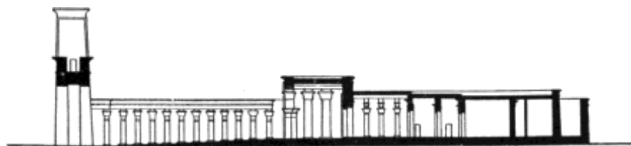
FIG. 10.—TEMPLE OF EDFOU. SECTION.
