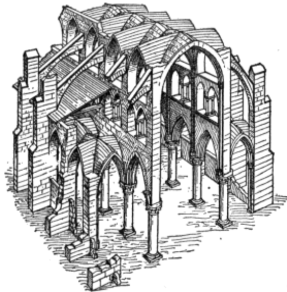
FIG. 105.—CONSTRUCTIVE SYSTEM OF GOTHIC CHURCH, ILLUSTRATING PRINCIPLES OF ISOLATED SUPPORTS AND BUTTRESSING.
