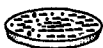
Porcelain disc used with Bunsen funnel to serve as semimicro suc- tion funnel
