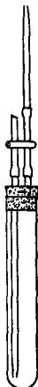
Separatory tube used in semimicro work in place of separatory or dropping funnel
