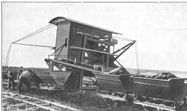
Abb. 39. Torfbagger Bauart Ekelund.
