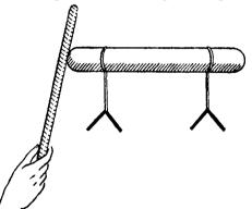
rubber rod is rubbed vigorously with the flannel and brought into contact with the metal. The leaves separate at once! They remain apart even after the rod is removed.
