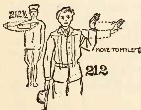
Fig. 212. Move to my left! Surveyors' signal which, reversed, would mean, move to my right. That this signal may be seen further, a surveyor sometimes holds a handkerchief in his hand and sometimes his hat in one hand and his handkerchief in the other.
