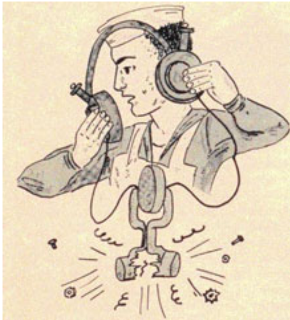
Figure 6-3. In case of casualty to the transmitter, speak into one earpiece and listen through the other.
