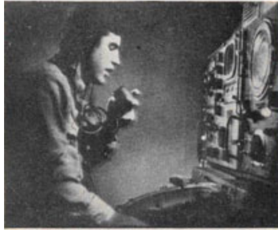
Figure 3-54. Reporting Jamming. "Bearing zero seven nine-range two-O double-O. Many fuzzy targets-looks like Window. Targets are stationary."
