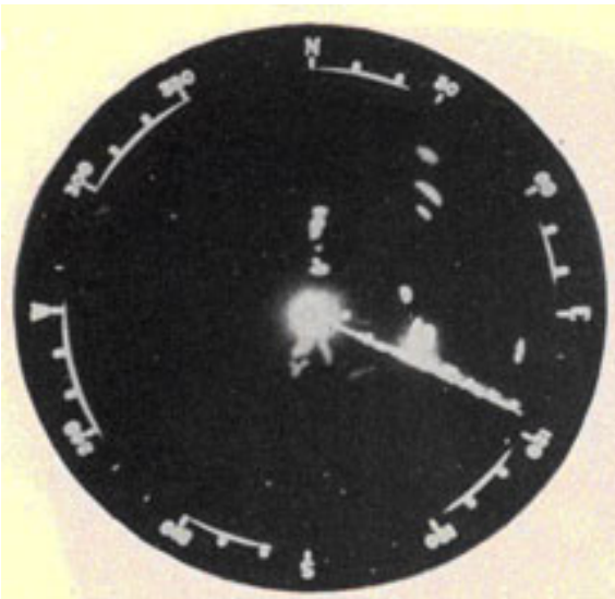
A. Aircraft at about half range, bearing 100 degrees true is about to sow Window to screen a destroyer, visible just beyond the plane.
