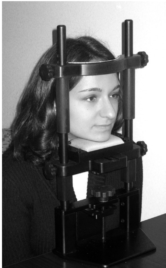
Figure 62.1 The EyeLink 1000 chin- and head-rest mount for head stabilization (and greater eye movement recording accuracy) while eye-tracking
