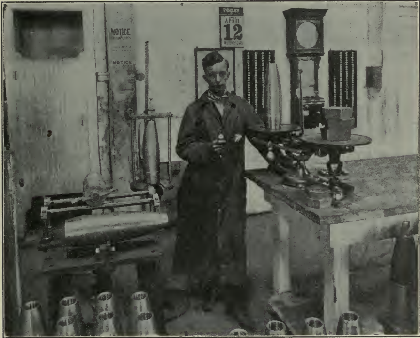
FIG. 396. TESTING SHELLS FOR ECCENTRICITY AND WEIGHT
