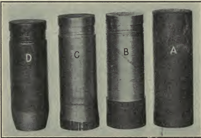
FIG. 178. THE ROUGH SHELLS (AFTER END IS CUT OFF) AND THE THREE FLAT-TURRET OPERATIONS
