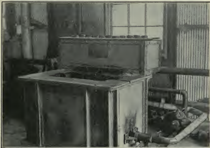
OPERATION 11. THE PREHEATING AND HEATING FURNACE
