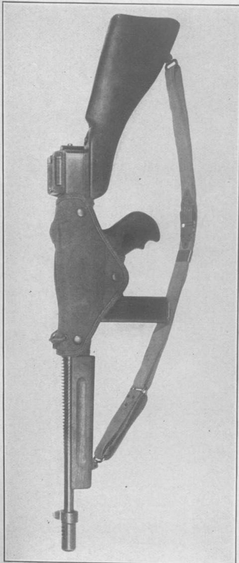
*Thompson Gun breach cover for the protection of gun mechanism—can be instantly taken off by one continuous pull on cover flap. After being detached in an emergency, a leather thong holds cover on gun so it will not be lost.*
