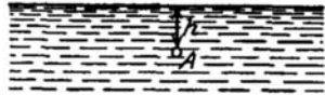
FIG. 59.—A fluid element in the interior of the fluid cannot reach the surface in a finite time (Lagrange's theorem).
