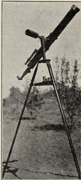
IRON TRIPOD MOUNT, Home-built, for 92 mm. Telescope.
