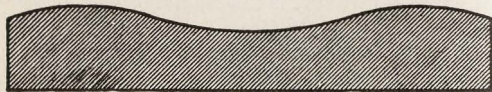
A cross section of the parabolized Mirror of comparatively short Focus. The depth of the curve of one of longer focus is very appreciably less.
