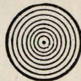
Diffraction rings surrounding star-image in a good objective, the ocular racked slightly out of focus.
