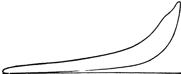
FIG. 132. Art. 306.— Indicator Diagram, Diesel Engine. (16 × 24 in. engine, 160 r.p.m. Spring 400.)
