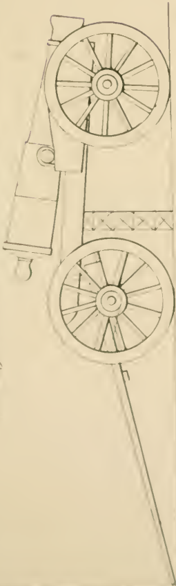
To change a limber when the piece is on its Travelling bed
